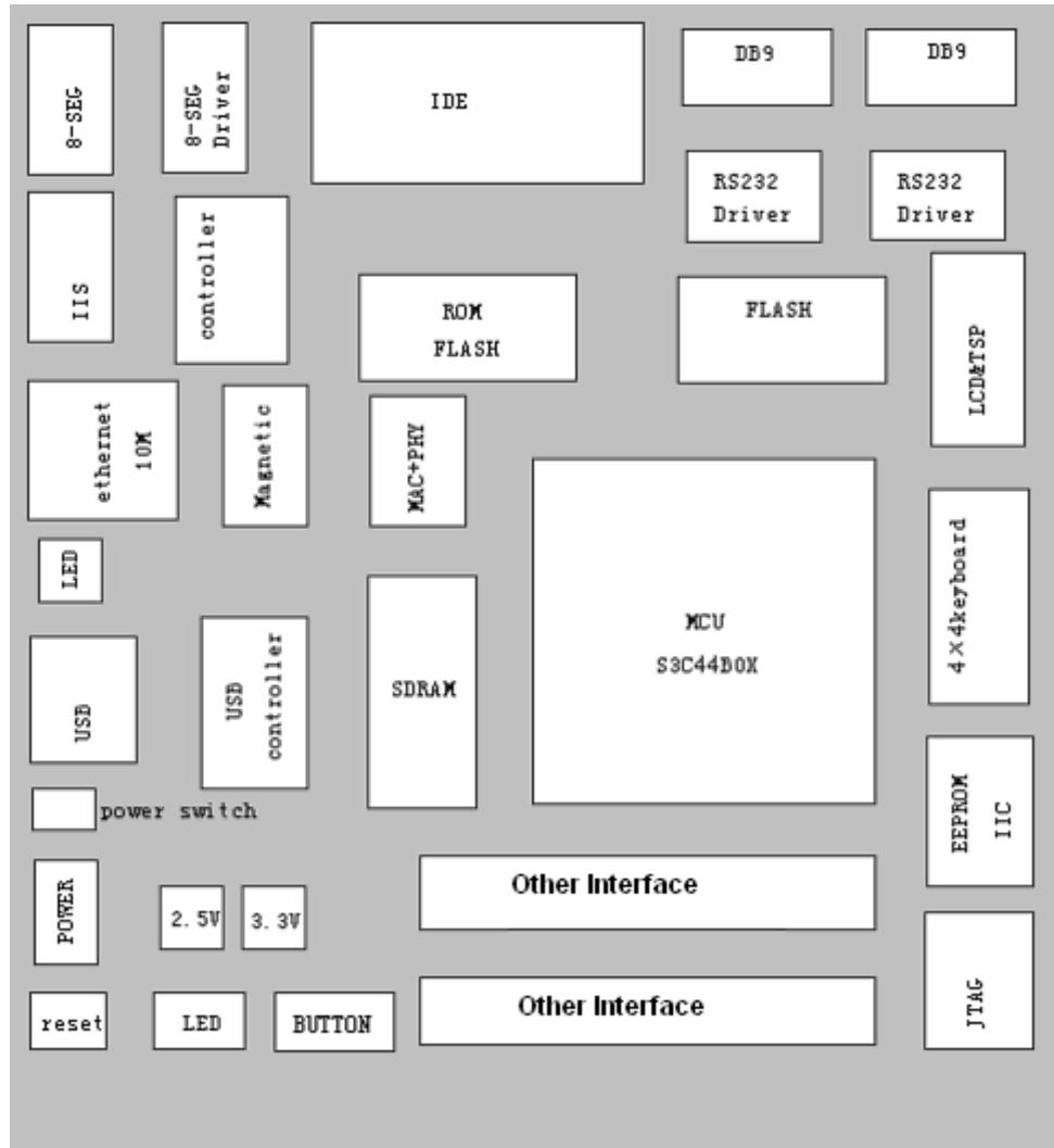
Figure 2-13 Embest S3CEV40 Function Block Diagram
